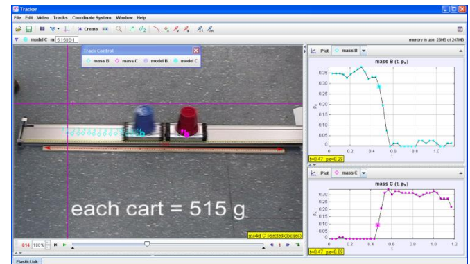
Figure 8. Use Tracker to analyze an elastic collision of a moving cart with a stationary cart of equal mass from Bryan’s website that shows the random errors in measurement of momentum px for both masses and the validity of conservation of momentum using velocities just before and just after collision.
