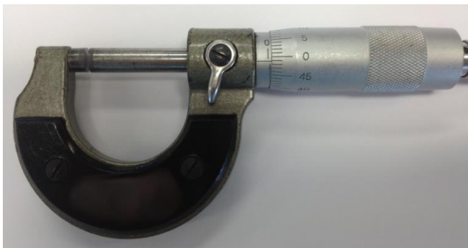
Figure 2. A micrometer used in the school and the reading is 0.99 mm.
