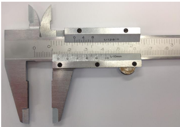
Figure 1. A vernier caliper used in the school and the vernier bottom scale spans 29 mm of the top scale. The reading is 14.2 mm.
