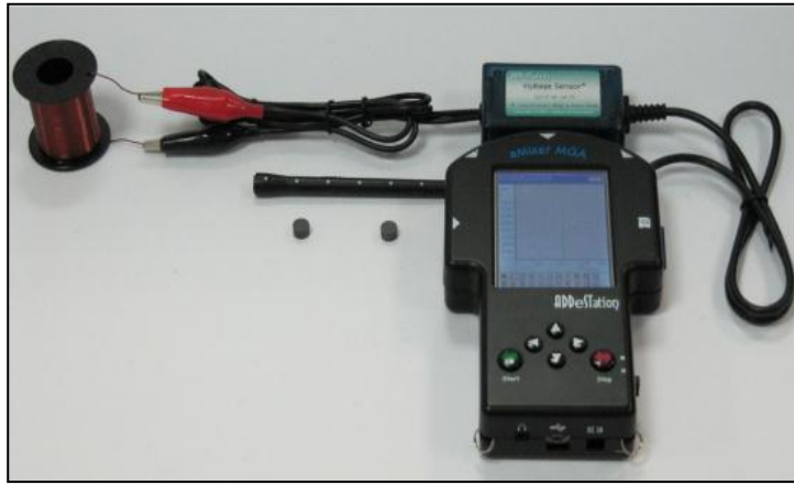
Figure 4: Data-logger apparatus for collection of data
